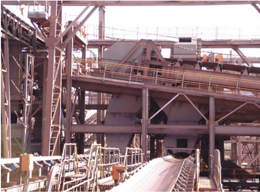
An example of a Weba chute in an iron ore application.
